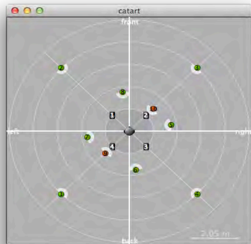
Figure 4. The surround panning space as it appears in the IRCAM spat user interface, in a 'bird's eye' perspective. The filled circles represent sound sources, and the squares represent outputs e.g. physical loudspeakers, or virtual sources for binaural reproduction.
