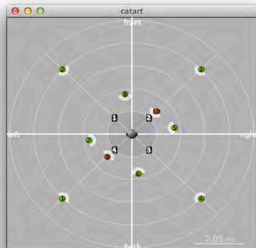
Figure 4. The surround panning space as it appears in the IRCAM spat user interface, in a 'bird's eye' perspective. The filled circles represent sound sources, and the squares outputs e.g. physical loudspeakers, or virtual sources for binaural reproduction.
