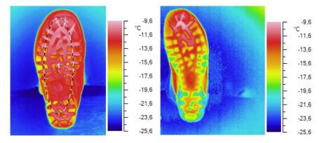
Figure 3. Termal images acquired at the end of the test for MODEL A (a) and MODEL B (b) both for Tester 1.
