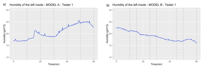
Figure 6. Humidity of the left insole for Tester 1 with MODEL A (a) and MODEL B (b).
