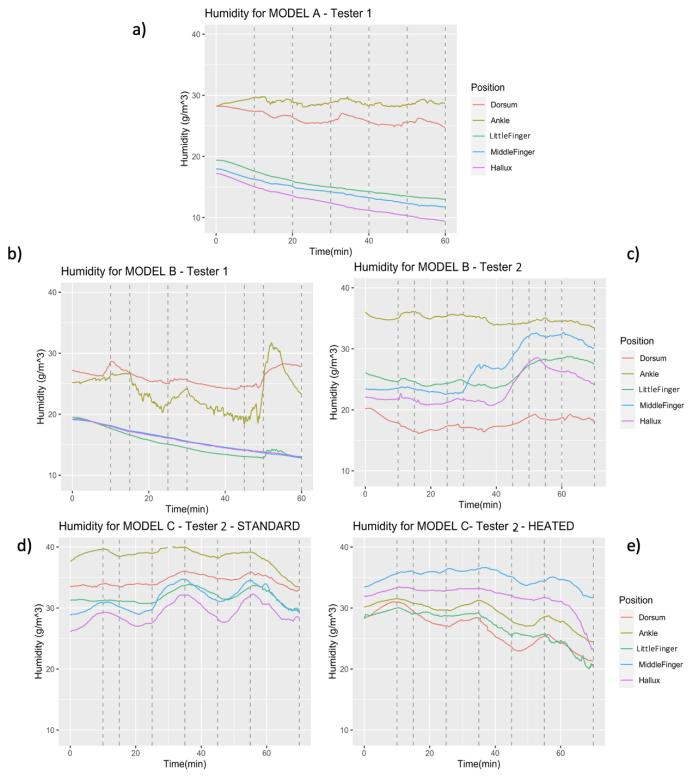
Figure 1. Humidity data for MODEL A (a), MODEL B for Tester 1 (b), MODEL B for Tester 2 (c), MODEL C without the heating system (d) and with the heating system (e).
