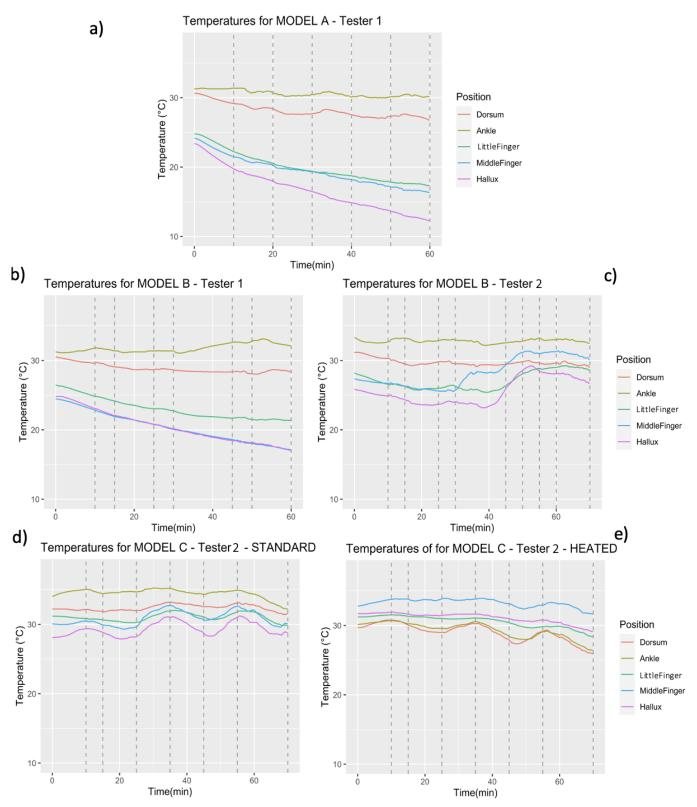
Figure 2. Temperature data for MODEL A (a), MODEL B for Tester 1 (b), MODEL B for Tester 2 (c), MODEL C without the heating system (d) and with the heating system (e).
