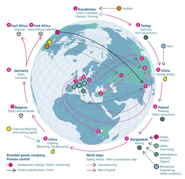
Fig. 2 The global value chain exemplifying the production of a cotton jeans (own illustration following [17]).
