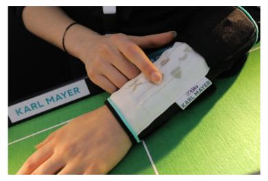
Fig. 5 Textile control panel
