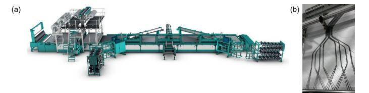
Fig. 3 (a) Example of a composite machine; (b) example of positioned carbon fibers in a non-crimp fabric
