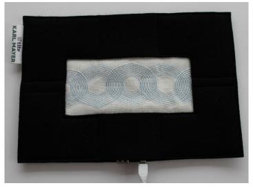
Fig. 4 Fully textile inductive charging pad
