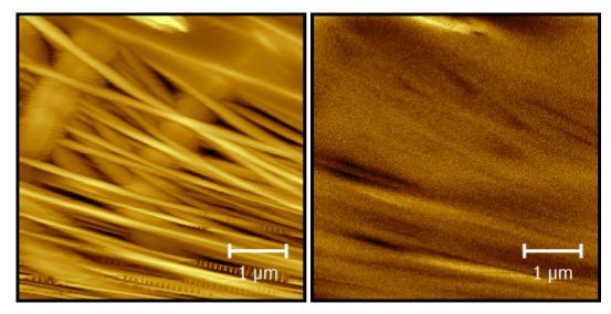
Fig. 5 (a) AFM topography image of a magnetically coated nanofiber mat; (b) MFM phase showing the magnetic properties of the sample (tip lift height 280 nm)
