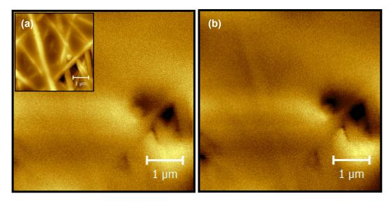
Fig. 4 MFM phases of a magnetically coated nanofiber mat with different tip lift heights: (a) 300 nm; (b) 240 nm. The inset shows the AFM topography.
