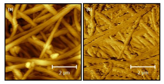
Fig. 2 (a) AFM topography image of a carbonized magnetic nanofiber mat; (b) MFM phase showing the magnetic properties of the sample (tip lift height 30 nm)
