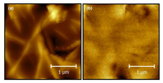
Fig. 3 (a) AFM topography image of a magnetically coated nanofiber mat; (b) MFM phase showing the magnetic properties of the sample (tip lift height 170 nm)
