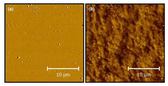
*Fig. 1 (a) AFM topography image of a magnetic thin-film sample; (b) MFM phase showing the magnetic properties of the sample*
