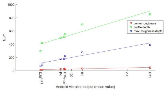
Fig. 7: Correlation between optical roughness and vibration output
