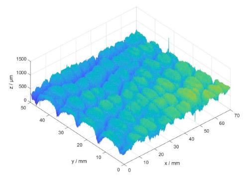
Fig. 3: 3D scan example of a textile surface
