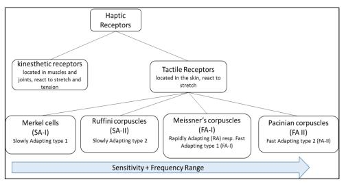
Figure 1: Classification of haptic sensors, following [7]
