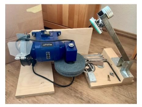
Fig. 1 A self-built test setup for testing the abrasion resistance of protective clothing.
