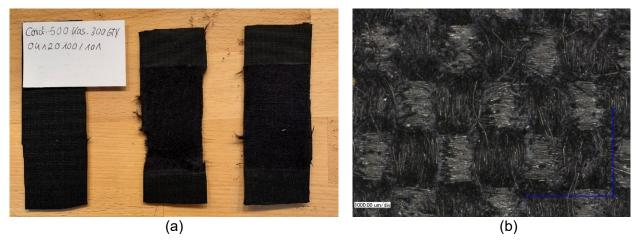
Fig. 5 The photograph and microscopic image of the CORDURA® 500 (laminated): (a) reference sample, damaged sample due to the impact simulation and sample after the abrasion test without a fall simulation; (b) microscopic image of the abraded surface.
