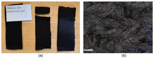
Fig. 4 Photograph and microscopic image of CORDURA® Air: (4a) reference sample, damaged sample due to the impact simulation and sample after the abrasion test without a fall simulation; (4b) microscopic image of the abraded surface.
