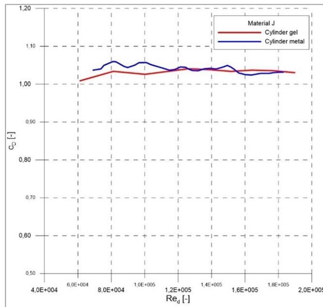
Fig. 7 Drag coefficient of soft-body cylinder with foil covered by material (J) and the rigid cylinder (metal).
