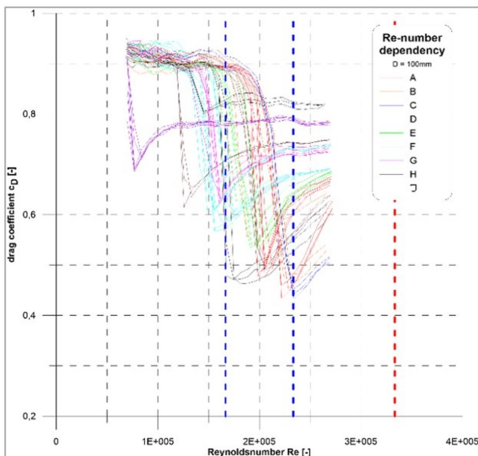
Fig. 2 Summary of drag coefficients behavior, measured for different textile materials covering rigid cylinders during the last years at the wind tunnel of TU Dresden.
