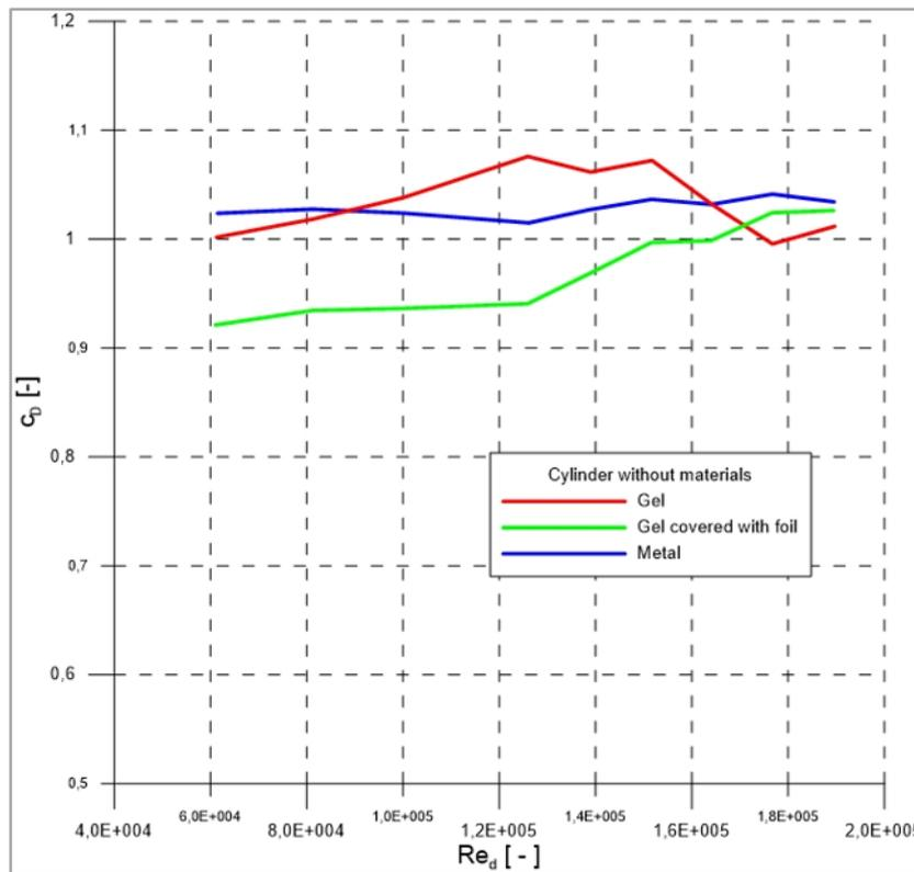
Fig. 5 Drag coefficient for cylinder with gel with and without covering foil and the rigid cylinder (metal), all without textile covering.
