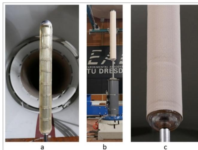
Fig. 4 Testing equipment for measurement of the drag coefficient at different Reynolds numbers in a wind tunnel: a) soft-body cylinder, b) with textile cover over the gelatin layer, c) close view of the cylinder with the textile.
