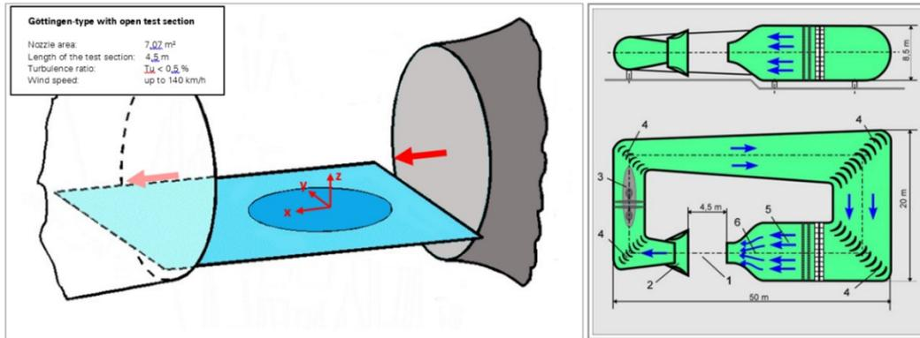
Fig. 3 Low-speed wind-tunnel Technische Universität Dresden, Chair of Flight Mechanics and Control.
