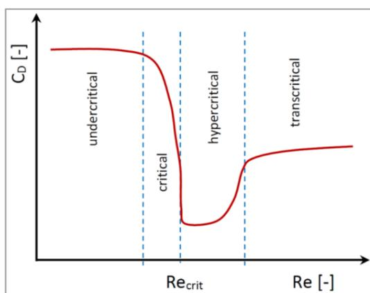
Fig. 1 Characterization of different areas of the resistance, following [6].
