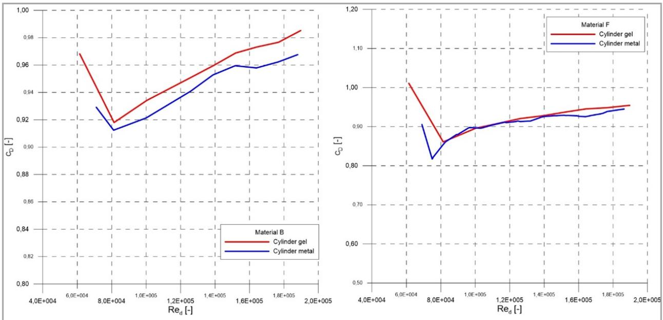
Fig. 8 Drag coefficient of soft-body cylinder with foil covered by two materials (B, F) and a rigid cylinder (metal).
