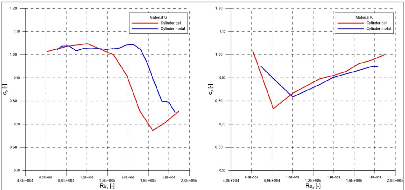
Fig. 6 Drag coefficient of soft-body cylinder with foil covered by two materials (G and K) and the rigid cylinder (metal).
