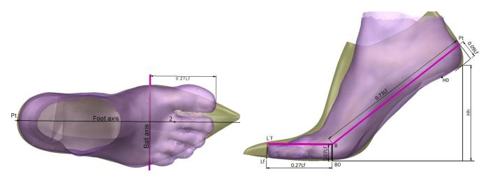
Fig. 4 Mutual alignment of the feet models for parameters comparison: a) top view and b) side view of the 3D foot and last models.
