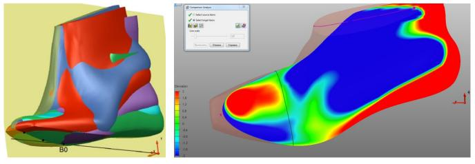
Fig. 8 Comparative analysis of the shoe last models in PowerShape CAD.
