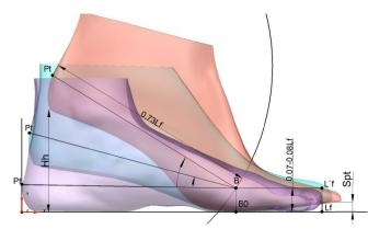
Fig. 5 Alignment of the last models with respect to the common coordinate system.
