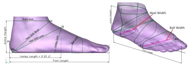
Fig. 3 Scheme of the foot measuring.
