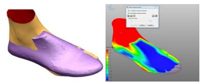
Fig.18. Comparison of the resulted shoe lasts with the customer's foot.
