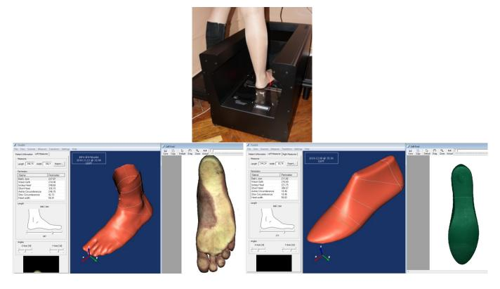
Fig. 1 Scanning process of the participants and 3D foot and last models in the Foot3D software.
