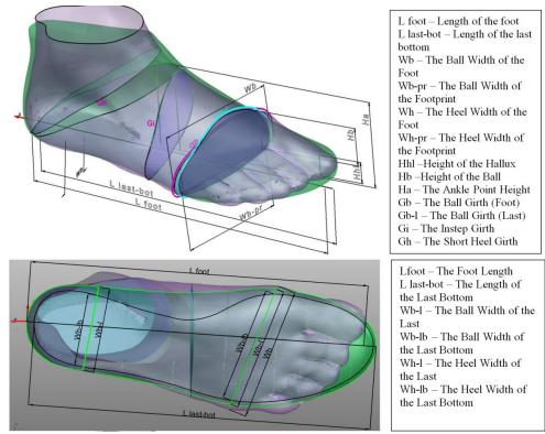
Fig. 6 Determination of basic foot measurements and shoe last parameters for comparison.
