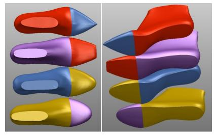
Fig.16 Variant of the extended range of last shapes resulting from the replacement of the toe part.
