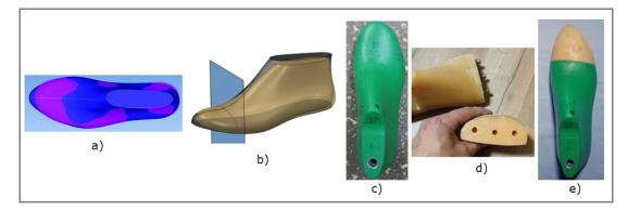
Fig. 17. The produced shoe last with a replaceable toe part: a) Comparison of the two 3D last models; b) section plane taken at last models; c) the last model of the first design; d) the second shoe last with the convertible toe part; e) the combined last shape.
