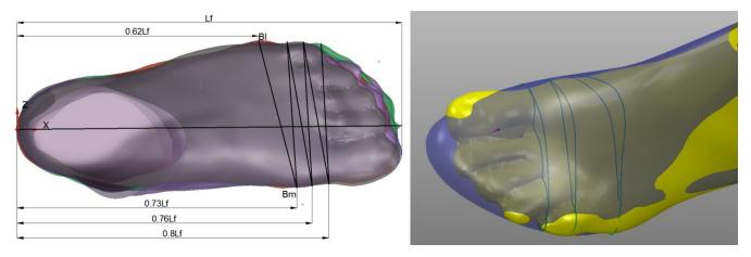
Fig. 9 Construction of cross-sections in the area of the search for a rational arrangement of the plane of last cutting.
