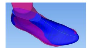
Fig. 13. Designing the shoe last shape in the mode of comparison with the foot
