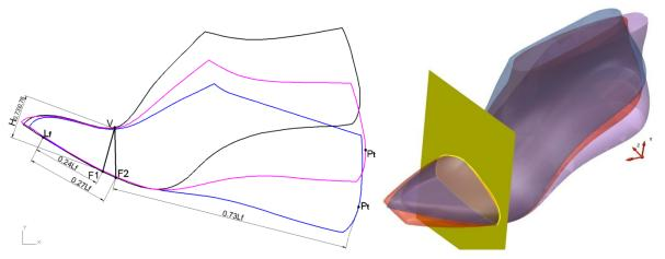
Fig.12 2D and 3D view of aligned lasts with a common sectional plane.
