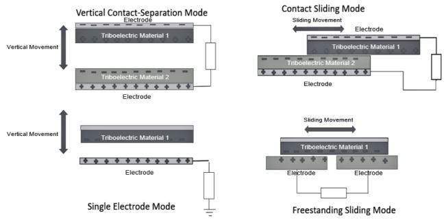
Fig. 1 Four fundamental modes of triboelectric characterization [17].
