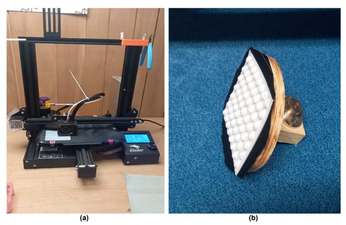
Fig. 3 3D printing on the textile substrate. (a) Filaflex is used to print on the textile substrate with flexible and elastic materials with a tensile elongation at break of 1400% (b) flexible, lightweight and soft 3D printed sample.
