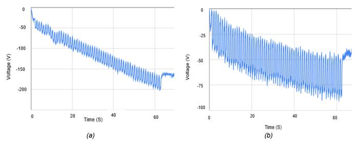
*Fig.* 5 Output voltages of the tapping and sliding mode of TENG: (a) tapping characterization voltage versus time; (b) lateral sliding characterization voltage versus time.
