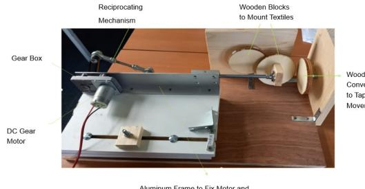
Wooden Block to Convert Device to Tapping Movement
