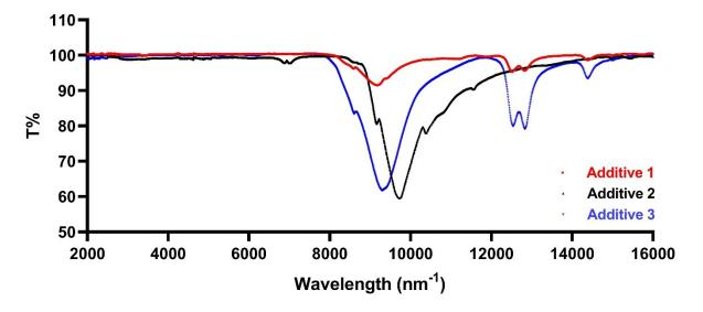
Fig. 1 Transmittance of three additives in the wavelength range from 2-16  $\mu$ m.
