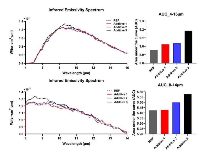
Fig. 2 Infrared emissivity spectrum of fabrics with inorganic additives in the ranges of 4-16 μm and 8-14 μm. The area under the curve (AUC) was calculated for each curve.
