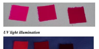
*Fig.* 6 Photographs of Rhodamine B containing cotton samples under different illumination (top: daylight; bottom: UV light). The Rhodamine B is applied on the fabrics from a solution containing water and iSys HPX in a ratio 1:1. The dye concentration is increased from left to right (0.5 wt-%; 1 wt-%; 3 wt-%).
