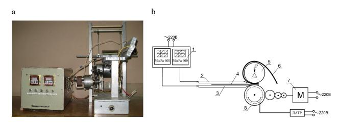
*Fig.1.* General view (a) and schematic diagram (b) of the laboratory installation for bonding of parts made of thermosensitive materials: 1 - temperature controller MikRa 600 upper (2) and lower (3) flat heater; 4 - sample of adhesive gasket material; 5 - upper calender; 6 – leather sample; 7 - engine; 8 - lower calender with heating.
