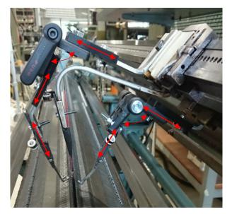
Fig. 6 Attachment of the modular yarn carriers to the knitting machine.
