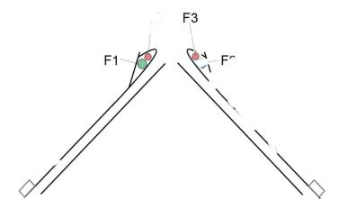
Fig. 3 Inserted yarns after lowering the needles; adapted from WO2020069856A1.
