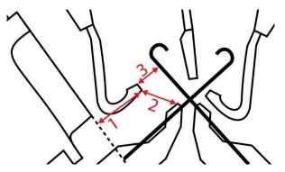
Fig. 7 The three different distances measured to define the exact positions of the yarn carriers.
