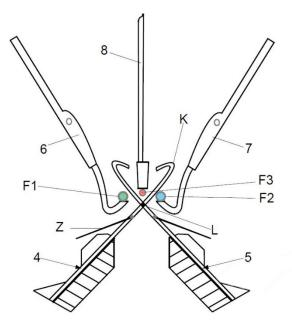
Fig. 1 Machine set-up for the realization of the innovative knitting technology; adapted from WO2020069856A1.
