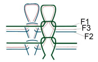
*Fig.* 5 The knitted structure of the innovative knitting technology resembles a knitted fabric plated from both sides; adapted from WO2020069856A1.
