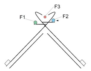
Fig. 2 Inserting the yarns into the needles at their maximum height; adapted from WO2020069856A1.
