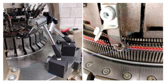
Figure 9 (a) The yarns F1 and F2 were fed to the needles using magnetic stand; (b) a first yarn F1 is inserted in the cylinder needles. A second yarn F2 is inserted behind the dial needles. A third yarn F3 is inserted into the dial and cylinder needles.
