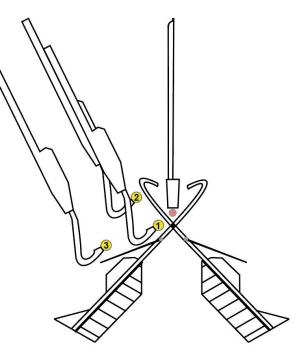
Fig. 8 Yarn carrier 6 is moved into three different positions to find the correct position; adapted from WO2020069856A1.
