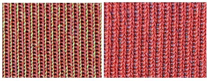
Figure 10 (a) Back side of the innovative knitted fabric. The red yarn is plated only on one side of the stitch so that the yellow yarn is still visible on the other half; (b) front side of the innovative knitted fabric. The red yarn is plated faultlessly so that the blue yarn is barely visible
