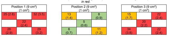
Position 1 has an average of 3 defects per cm<sup>2</sup>. Position 2, on the other hand, has a significantly lower defect rate with an average of 1 defect per cm<sup>2</sup>. Position 3 is in the middle range with an average of 2.5 defects per cm<sup>2</sup>. It can be concluded that position 2 produces results with the lowest defect rate and is therefore the most suitable position.
