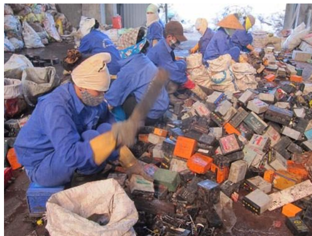
Figure 2. The workers were extracting Pb from fail batteries
