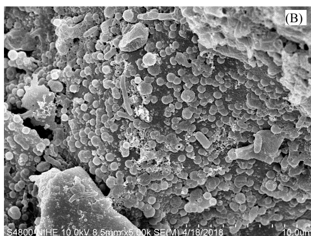
Fig. 4. Scanning electron microscopic (SEM) images of the biocarriers without the bacteria (A) and with the consortium colonizing the surface of the biocarriers (B).
