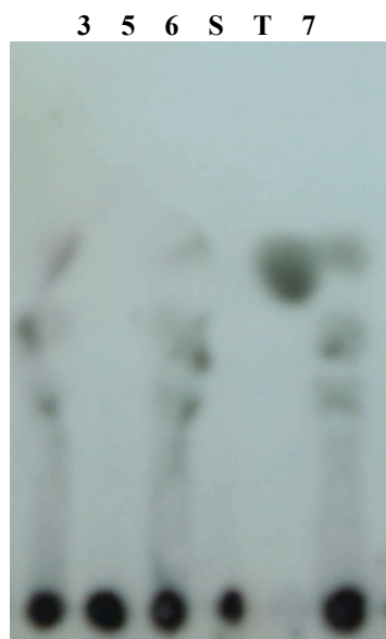
Figure 2. Visualization of MTSase and MTHase catalysis reaction products by TLC (3: DT1 ; 5: 91 ; 6: DN 4 ; 7: P. putida ; S: starch, T: Trehalose)
