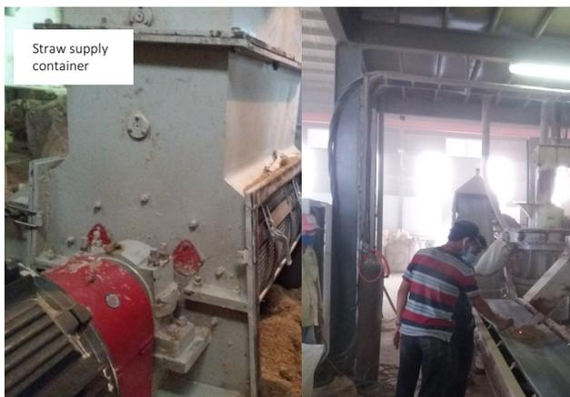
Figure 5. Rice husk grinding machine
