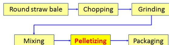
Figure 2. Straw pelletizing process from straw bales
