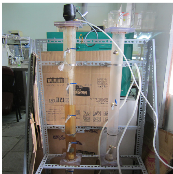
Figure 2. Schematic diagram of UV/O 3 apparatus
