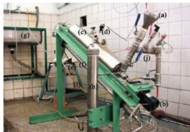
Figure 4. Photo of the CHTC bench-scale reactor setup
