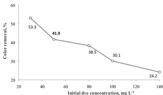
Figure 6. Effect of dye concentration on EC of the dye (SO<sub>4</sub><sup>2-</sup> 1200 mgL<sup>-1</sup>, pH 11, *i* 3 A, and *t* 4 min)
