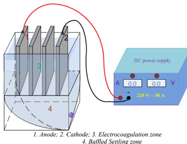
**Figure 2. Bench scale of the EC reactor**
