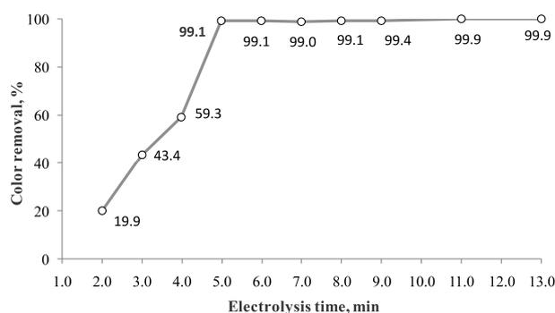
Figure 8. Effect of electric current on color removal efficiency (SO<sub>4</sub><sup>2-</sup> 1200 mgL<sup>-1</sup>, pH 11, IDC 50 mgL<sup>-1</sup>, and *i* 4 A)
