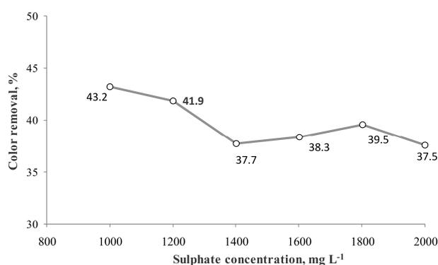
**Figure 5. Influence of sodium sulfate concentration on dye color removal (IDC 50 mgL<sup>-1</sup>, pH 11, *i*3 A, and *t* 4 min)**
