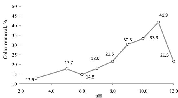
**Figure 3. Effect of initial pH on color removal efficiency (IDC 50 mgL<sup>-1</sup>, SO<sub>4</sub><sup>2-</sup> 1200 mgL<sup>-1</sup>, *i*3 A, and *t* 4 min)**
