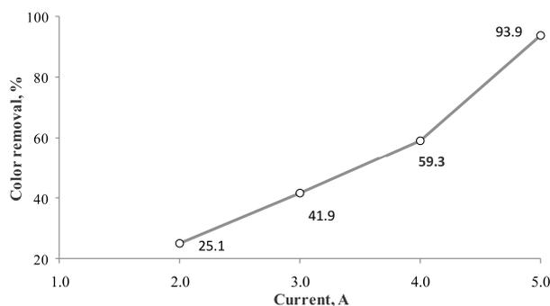
Figure 7. Effect of electric current on color removal efficiency (SO<sub>4</sub><sup>2-</sup> 1200 mgL<sup>-1</sup>, pH 11, IDC 50 mgL<sup>-1</sup>, and *t* 4 min)
